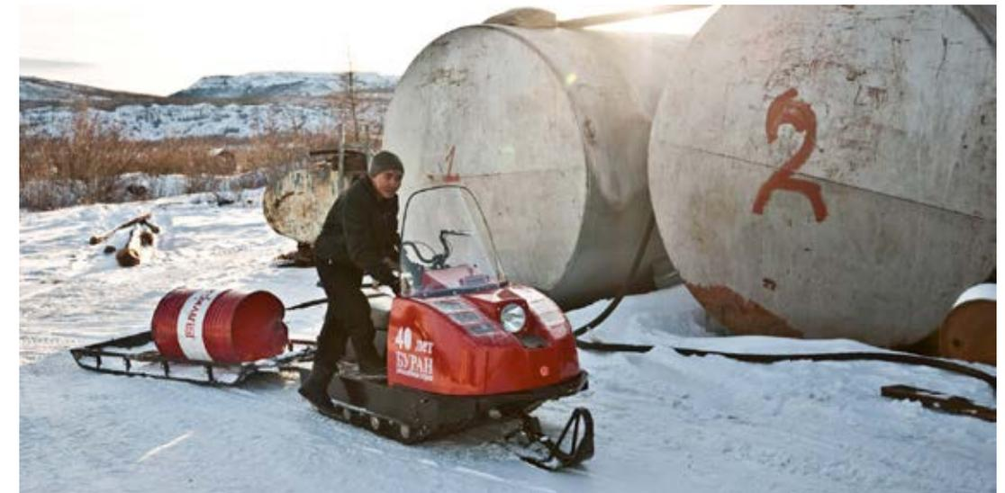
The dual-track snowmobile “Buran” has been produced in Russia for over 40 years. The design of the “Buran” has remained almost unchanged since it first came off the assembly line. This snowmobile is the hunter’s favoured mode of transport and local villager’s main means of communication.
